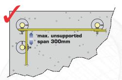
Unsupported spans of KGUARD barrier should not exceed 300mm. Always use two K2 Socket Bases at corners.
