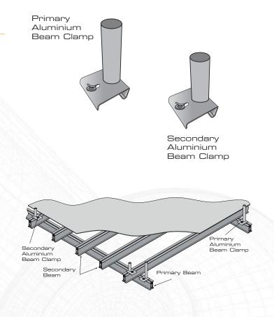
Note: Ensure formwork has been correctly assembled to manufacturers specification and all beams are correctly assembled together. All Aluminium and Timber Beam Clamps must be at least 150mm in from the end.
