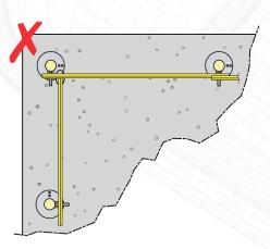
Do not use temporary ties to join an unsupported span to another barrier at a corner. Each panel must be supported by two KGUARD Support Safety Posts.
