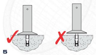
Thread the K2 Socket Base into the anchor until the bottom is touching the concrete.
